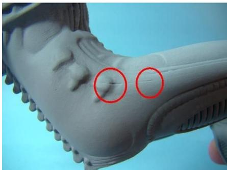
The primer coat on this figure revealed areas where the seam was still visible – marked with the red circles).
